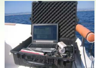
Sealed box where are inserted the computer, the USR-96, the GPS, and all the connections.
